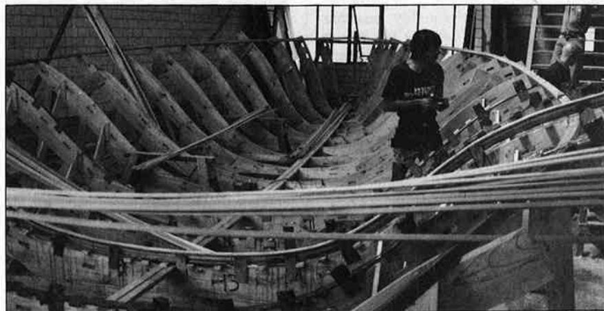
Female jig assembled with laminated cedar/ash frames being made up.
