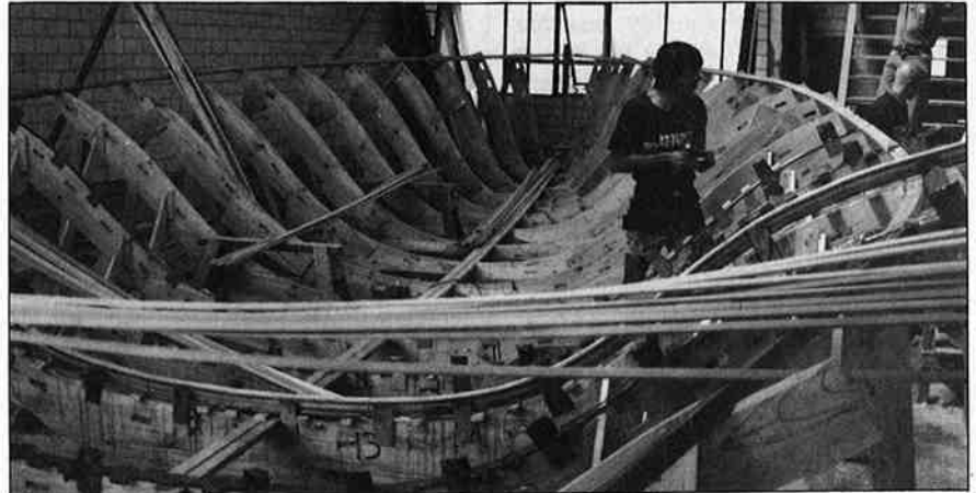
Female jig assembled with laminated cedar/ash frames being made up.
